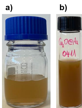
Figure 19. Synthesis of Cu 2 O@Au. The as synthesised heterostructured NPs (a) before and (b) after the purification.
